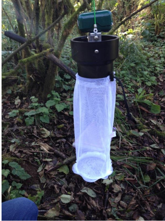
Photo 2. CDC light trap hung from a tree limb to collect adult mosquitoes at the SFC site, 2015.
