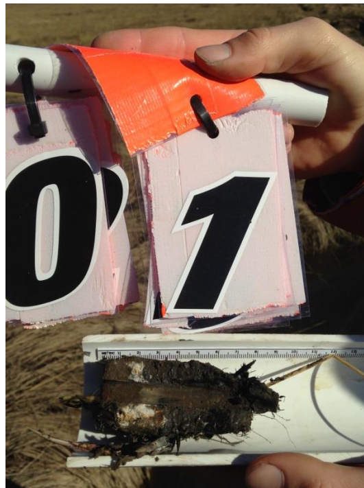
Photo 1. Example of field photo showing a feldspar marker horizon core and its sample number. A photo like this was taken of each core, for archival purposes. Sediment to the left of the white feldspar marker horizon has been deposited over the past year.
