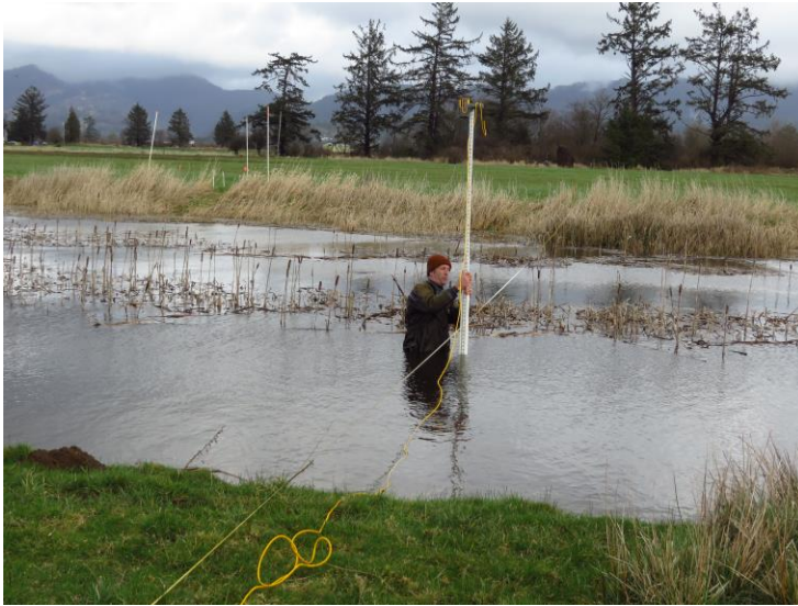
Figure B18. Stan van de Wetering, CTSI, measuring channel cross-sections in Nolan Slough with the laser level. Photo by Laura Brophy.
