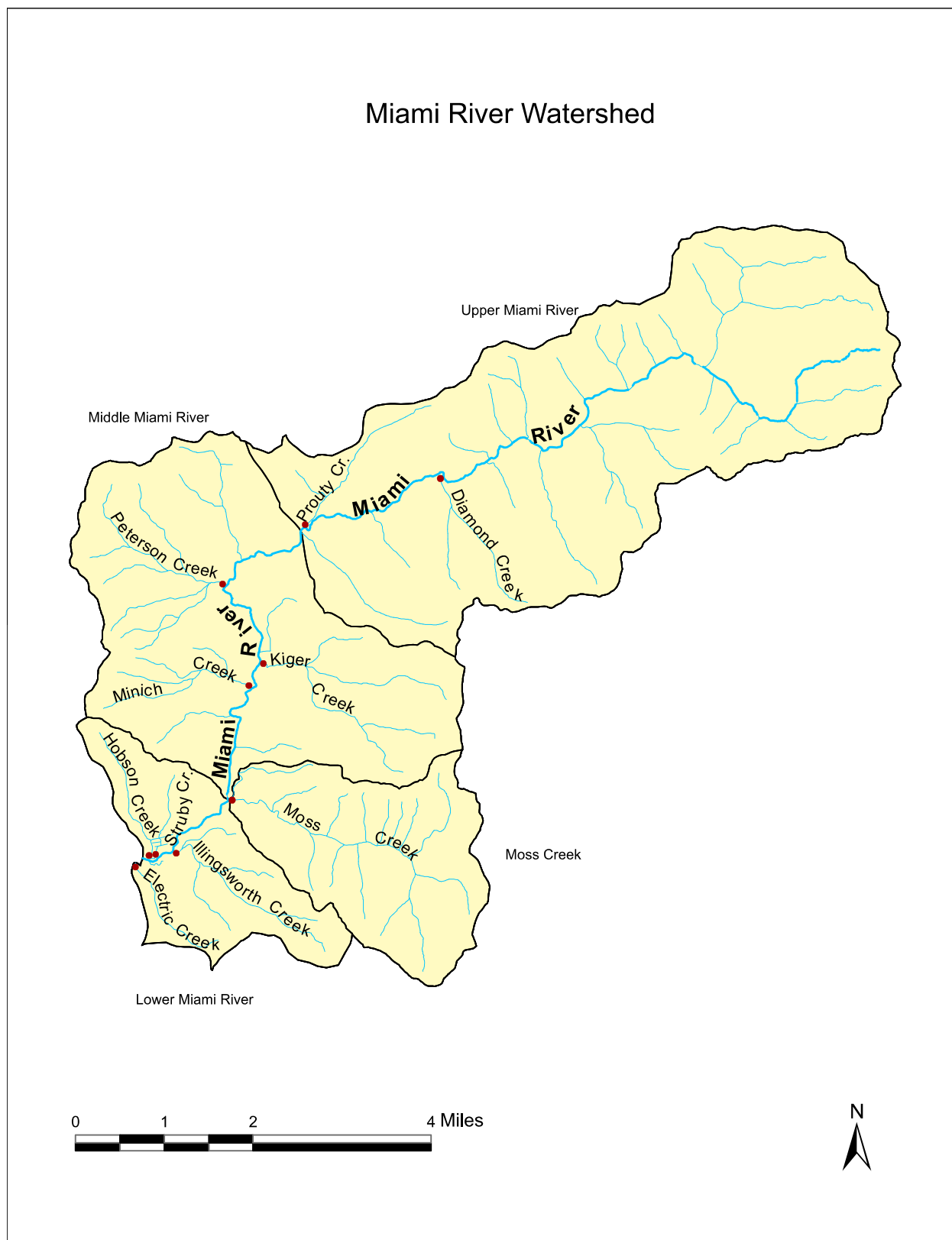
Figure 1.2. Map of Miami River watershed showing subwatershed boundaries and stream network, with names of streams indicated.
