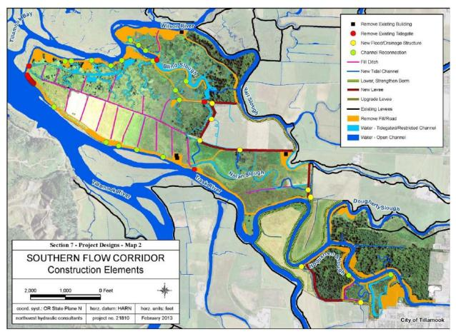
Figure 2. SFC project area: Construction elements
