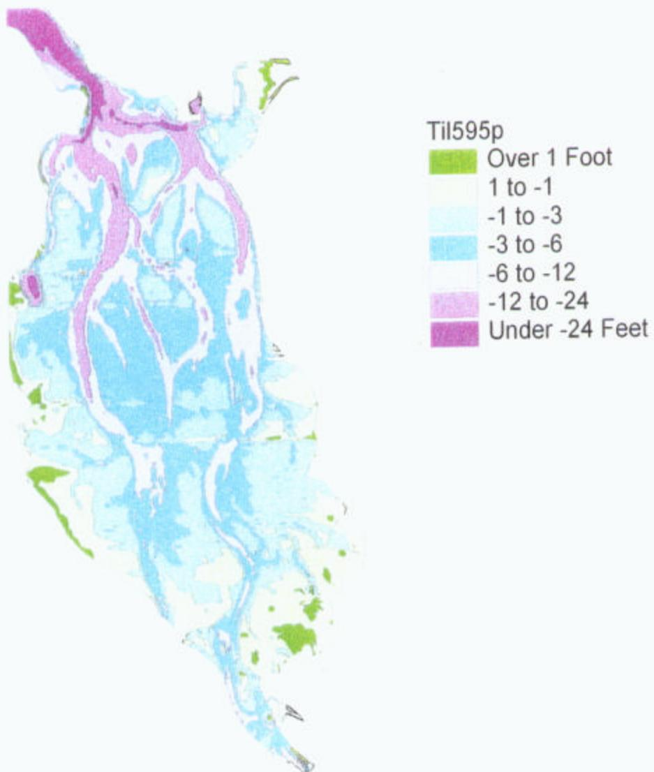
**Figure 5.** Bathymetric surface derived for 1995.
