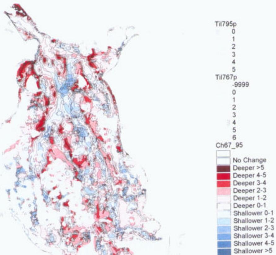
Figure 10. Cumulative change analysis for overall period 1867 to 1995, as shown in Figure 9, except that areas are represented in grey tone where the kriging variance was greater than 2 ft.
