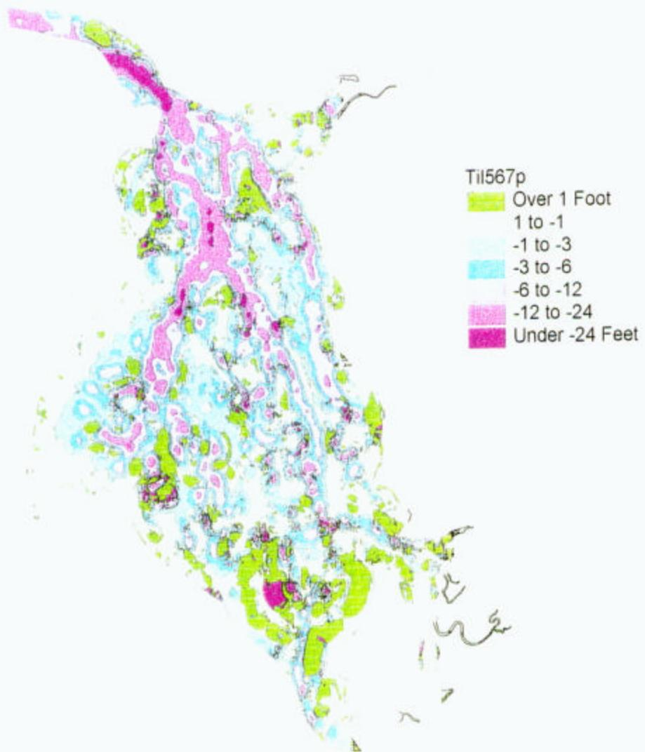
Figure 3. Bathymetric surface derived for 1867.
