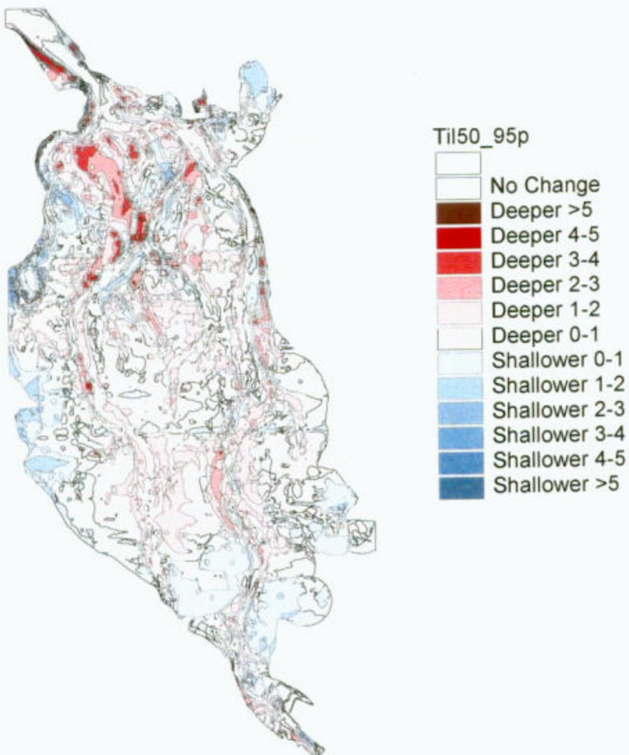
**Figure 8.** Inferred change in bathymetry from 1957 to 1995. No correction has been made for differences in benchmark elevation (datum shift) or sea level rise. Such corrections would change the inferences depicted here by an unknown amount.
