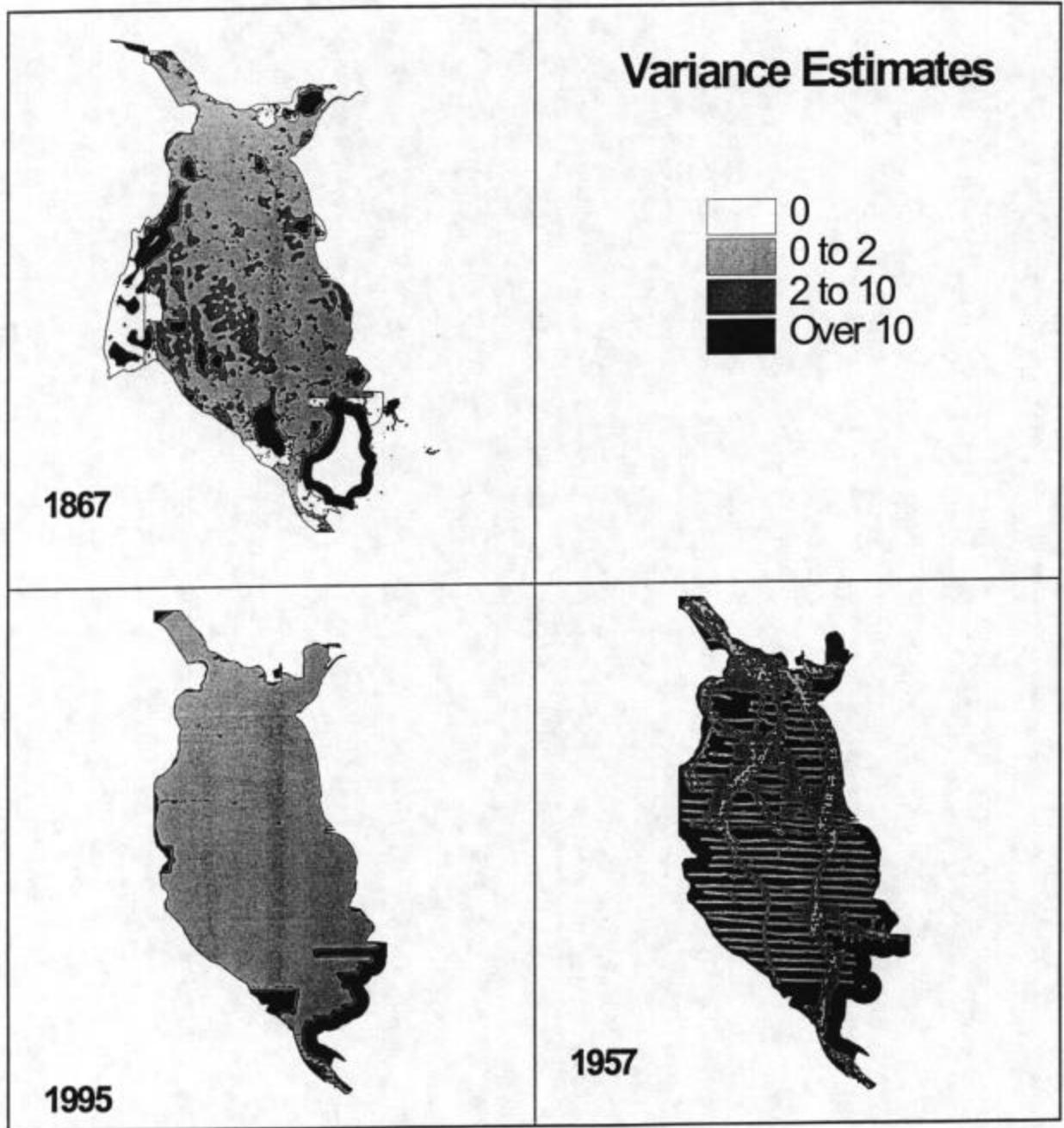
**Figure 6.** Variance in the interpolation methods for 1867 (a), 1957 (b), and 1995 (c). Note that this does not represent the total variance in the modeled (mapped) bathymetry. It only includes the portion of the variance that is associated with the kriging algorithm. Other important sources of variance are measurement errors, including the ability to standardize measurements to the tidal fluctuations. The latter were undoubtedly much larger in the earlier surveys.
