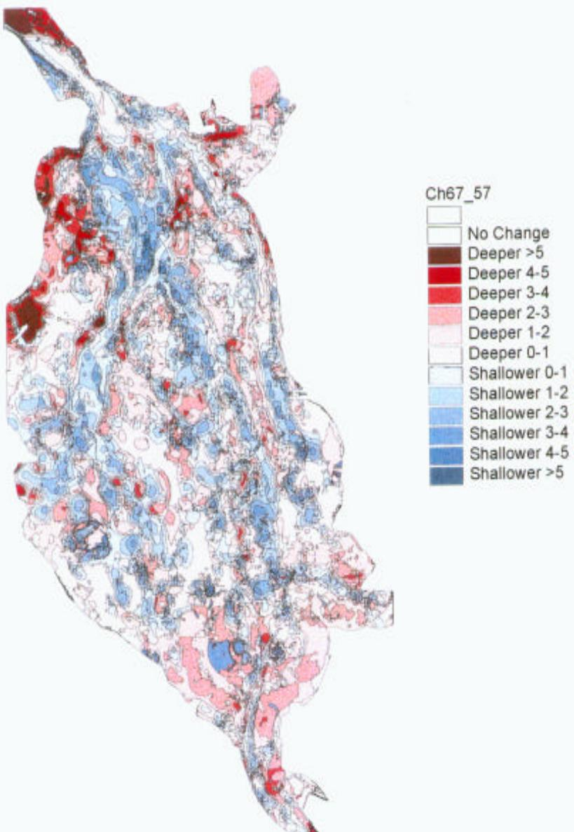
**Figure 7. Inferred change in bathymetry from 1867 to 1957.** No correction has been made for differences in benchmark elevation (datum shift) or sea level rise. Such corrections would change the inferences depicted here by an unknown amount.
