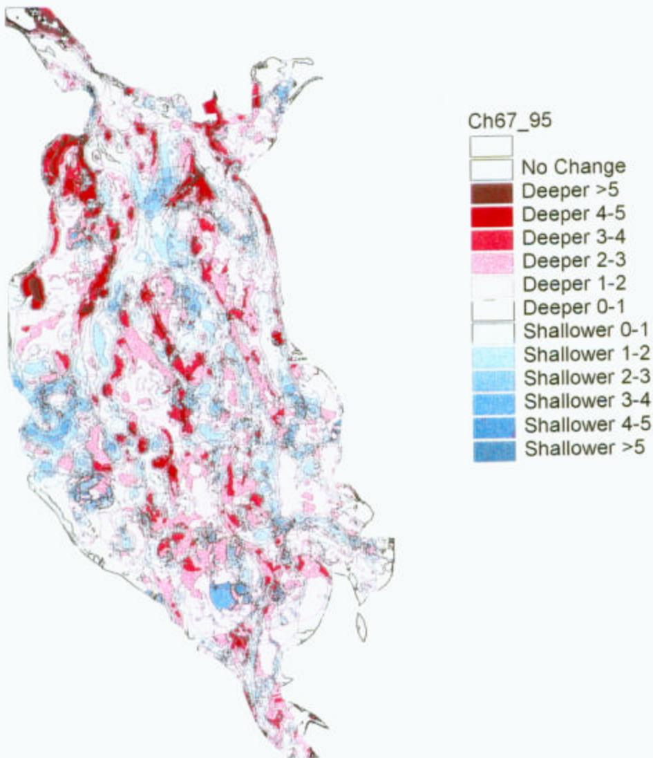
**Figure 9.** Inferred change in bathymetry from 1867 to 1995. No correction has been made for differences in benchmark elevation (datum shift) or sea level rise. Such corrections would change the inferences depicted here by an unknown amount.
