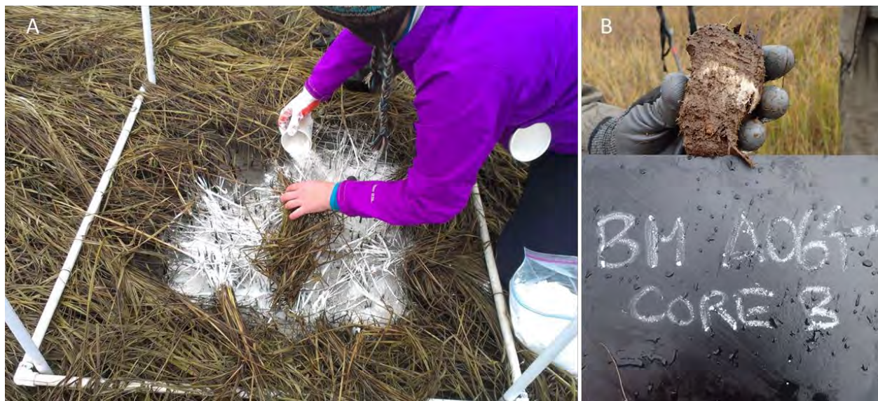
Figure 2.3. (A) Establishment of a fieldspar marker horizon layer inside a 1.0 m 2 plot in 2013, and (B) example of a sediment wedge collected in 2018 to measure accretion 4.9 years after plot establishment. Photos by C. Janousek.
